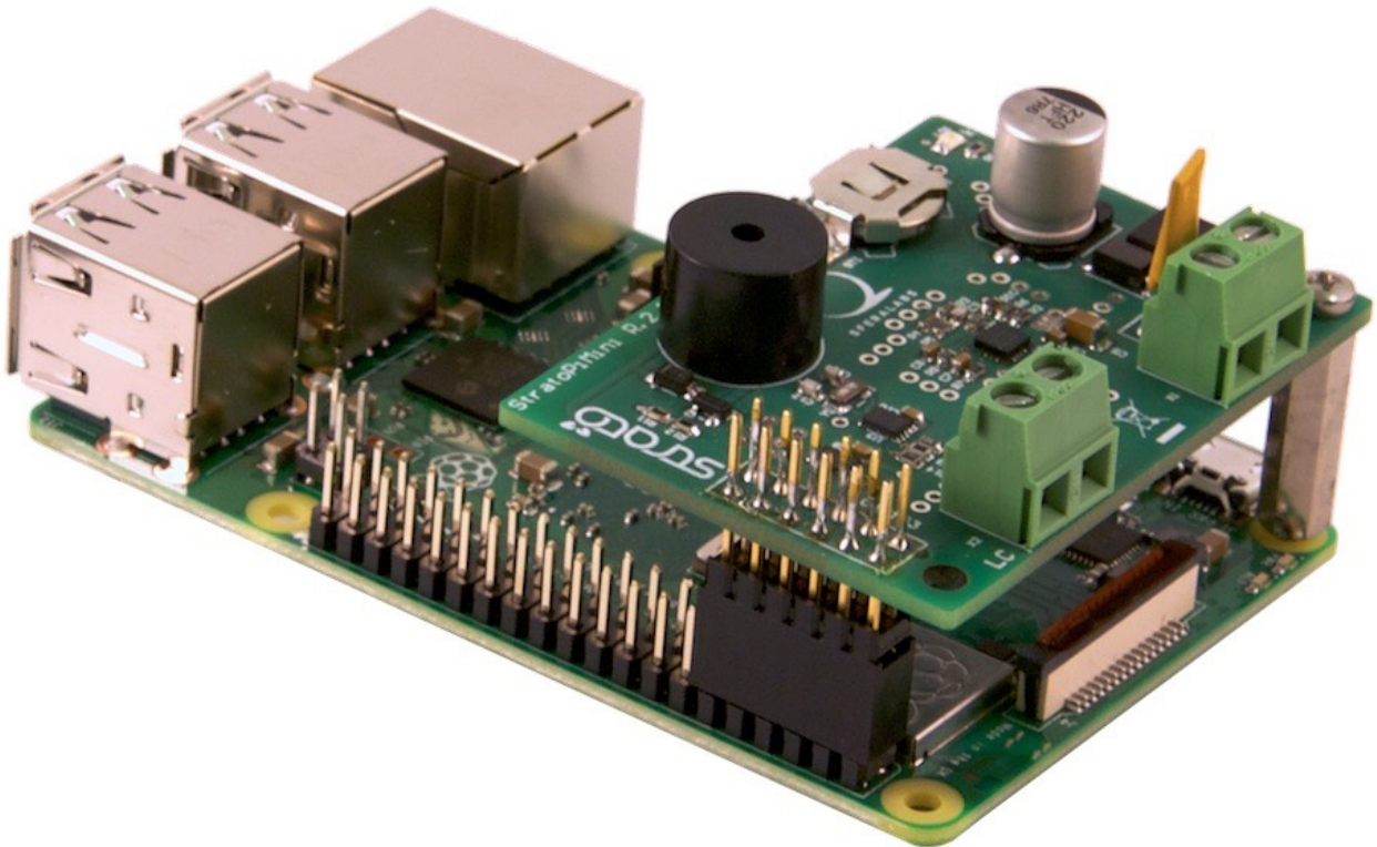
STRATO PI MINI BOARD INSTALLED ON THE RASPBERRY PI
