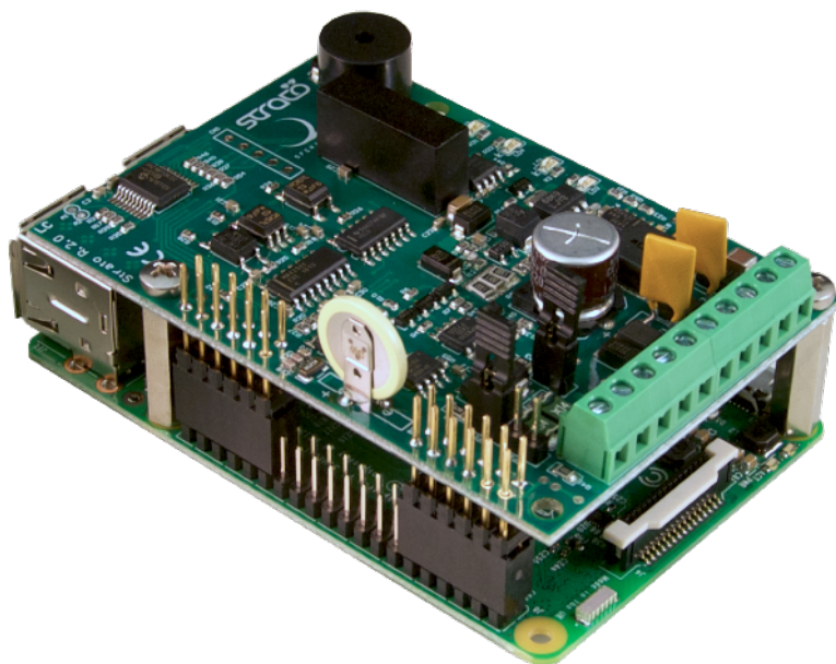
STRATO PI UPS BOARD INSTALLED ON THE RASPBERRY PI
